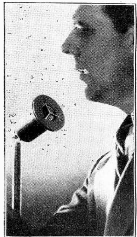
DIRECTIONAL OR NON-DIRECTIONAL. This versatile microphone, produced by the American Western Electric Company, may be converted from a highly directional instrument, relatively insensitive to extraneous noises, into one having a good all-round pick-up. The conversion is made by removing the disc "baffle" cover.
