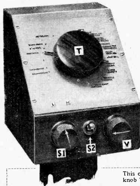
Fig. 1.—The signal-frequency tuning system is shown here. T1 and T3 are the aerial-to-line and line-to-receiver matching sections, and T2 is the tuning circuit in the control unit.
