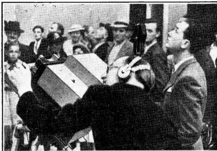
PARIS FOLLOWS LONDON. Impressed by the successful transmission of outdoor scenes by television in this country, the French Broadcasting Authorities are carrying out similar experiments. It will be noticed that an E.M.I. Emitron camera is being used.
